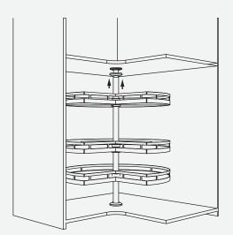
4. Adjust the actual height and fixing top plate and cover it.
