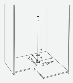
1. From central postion to back panel : 370mm Fixing the bottom panel and cover it
