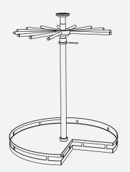
3. Fixing layer of hanger: a. Plate (Fixed by 5mm pin); b. Hangers;
