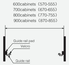
2. Cover of the slide rail is arranged on the slide rail pad from top to bottom
