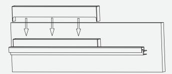
3. The frame from the top down on both sides of the slide. Note that the front of the frame should be attached to the front of the slide rail.
